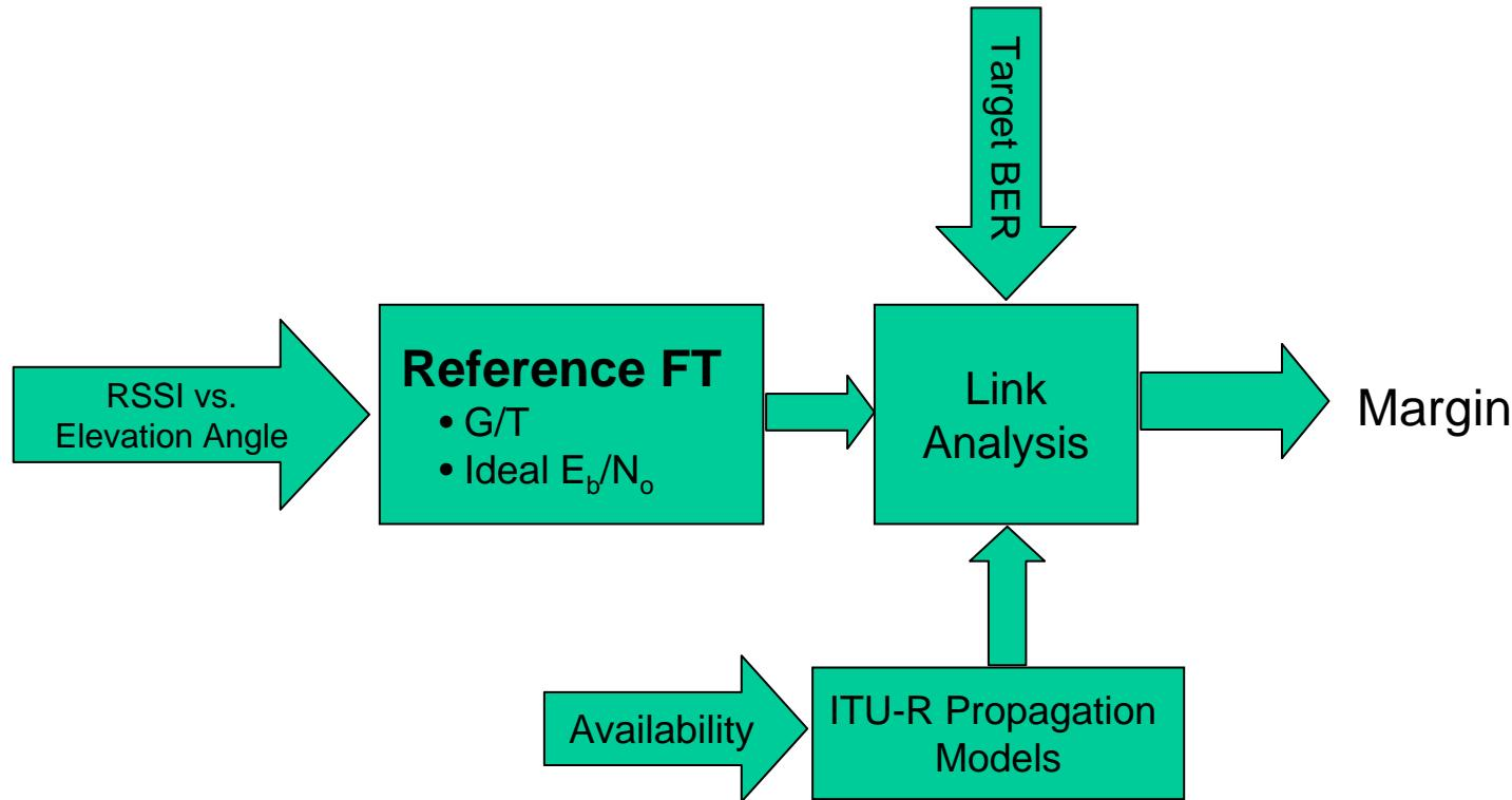
Orbit-Average Availability Calculates the Availability That Zeros the Margin at Each Elevation Angle and Weights the Availables by the Probability of Being at Each Elevation Angle
