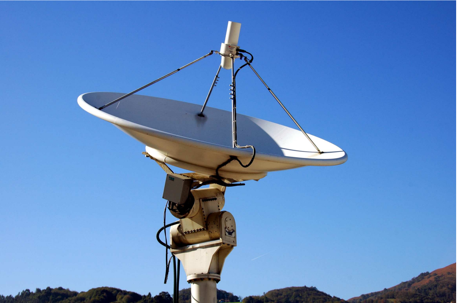
Figure 1: Antenna MODIS at the University of Oviedo (Diameter = 2.4 m).
