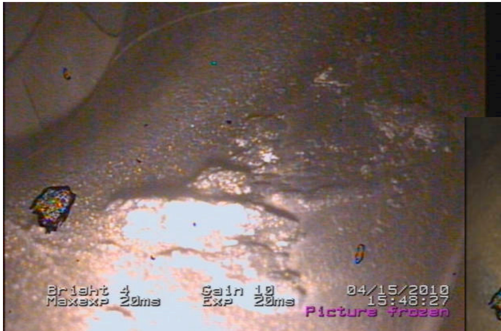
Melted quarts/ash in F18 Hornet engine. Finnish Air Force, 2010.
